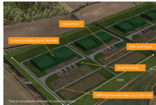
3D visualisation of project substation (HVDC option)
